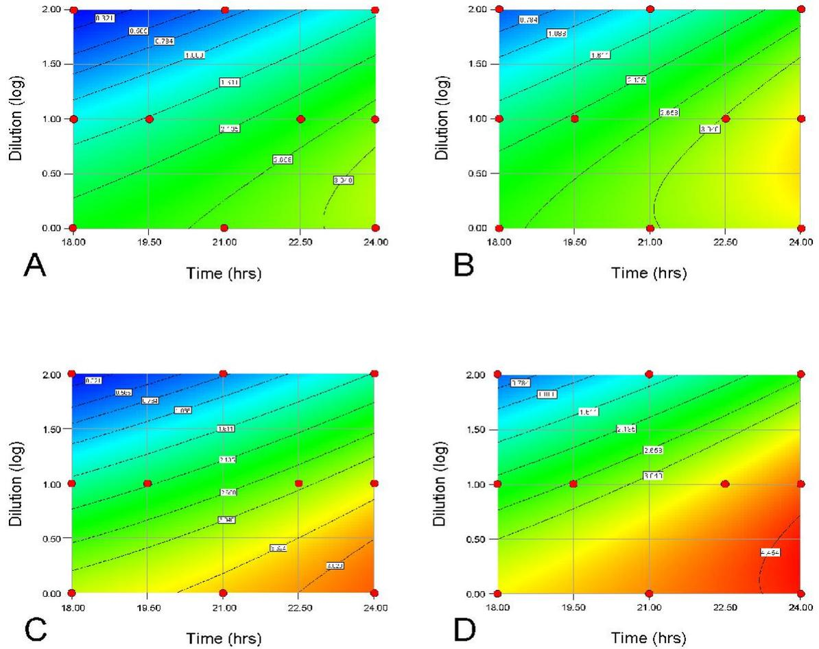
**Figure 2.** OD<sub>600</sub> time x dilution contour plots for *Agrobacterium* culture density in un baffled and baffled flasks. A) un baffled flask at 26C; B) un baffled flask at 28C; C) baffled flask at 26C; D) baffled flask at 28C. Dilution was in logs but coded as 0 = 1/10, 1 = 1/100, and 2 = 1/1000.
