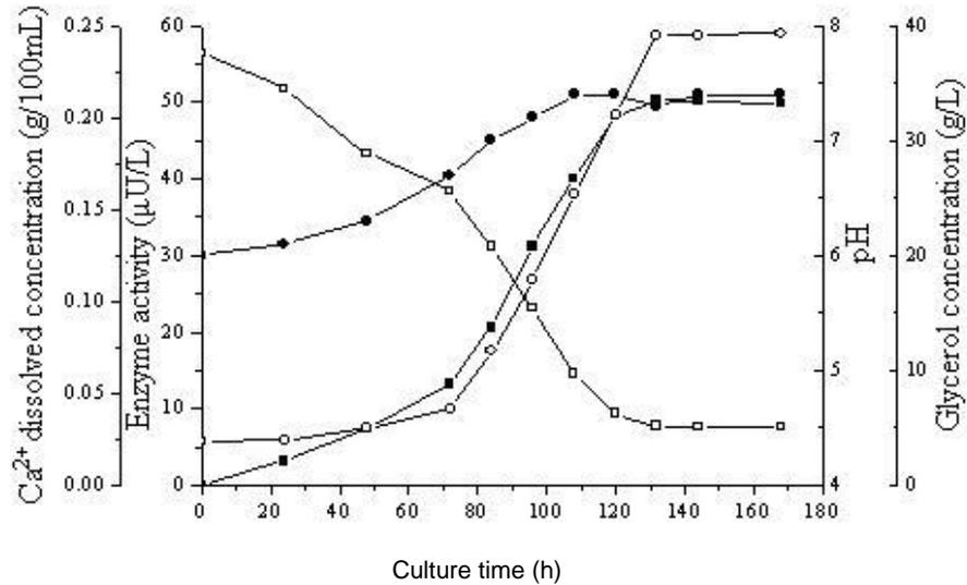
**Figure 2.** Typical curve of *B. mucilaginosu* K02 cultured in medium for carbonic anhydrase synthesis supplied with 7 g/L limestone. Ca<sup>2+</sup> dissolved concentration (○), CA production (■), glycerol consumption (□) and pH (●) by *B. mucilaginosu* K02 in a 5-L B. Braun Biostat Q fermenter.
