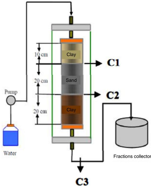
Figure 3. Set-up used for the column experiments.
