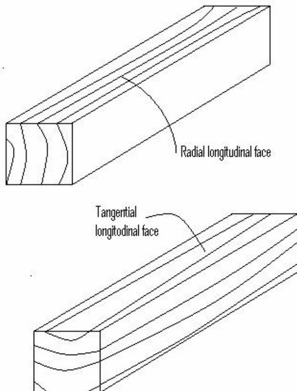
**Figure 1.** Radial and tangential face hardwood specimens (Drawing not to scale).
