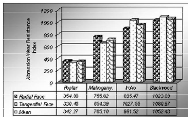
**Figure 3.** Abrasive-wear resistances of hardwoods on radial and tangential faces.
