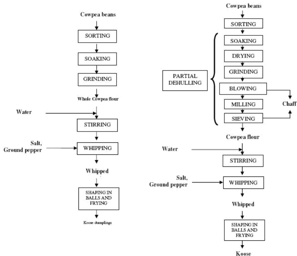
Figure 4. Flow diagrams for koose processing.
