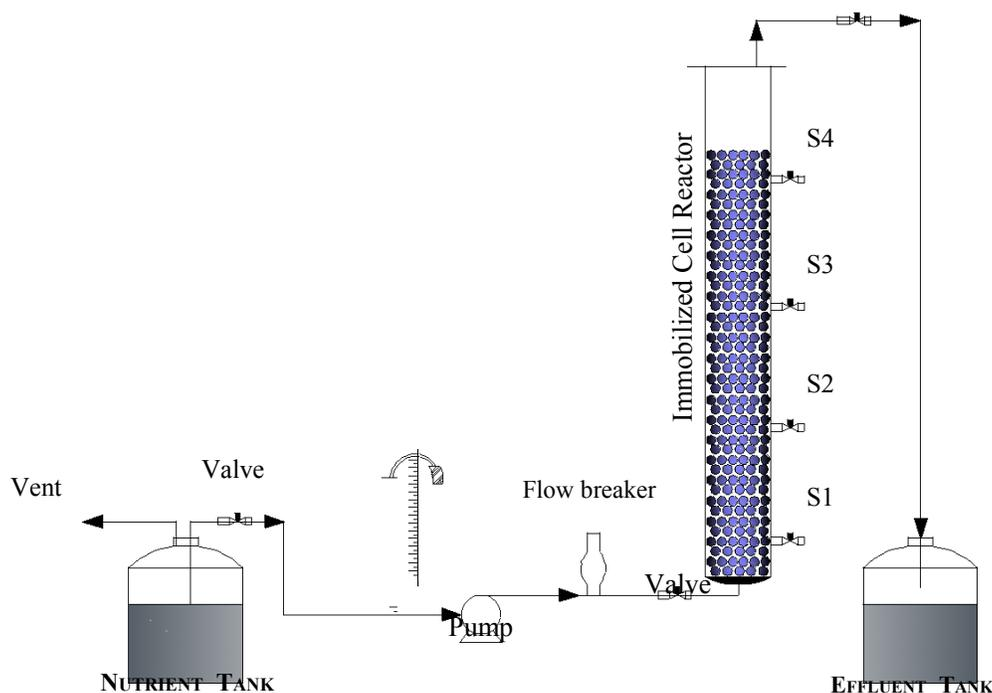
Figure 1. Schematic diagram of ICR experimental setup.
