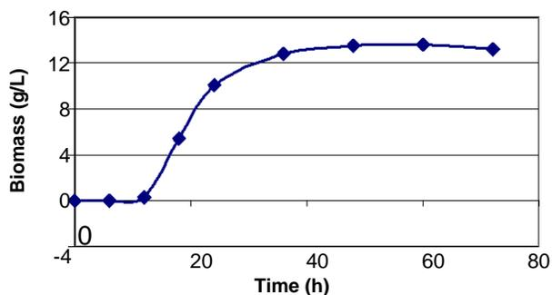
**Figure 1.** Shows the rate of production of fungal biomass during lipase fermentation by *Trichoderma viride* at  $30\pm 1^\circ\text{C}$ .
