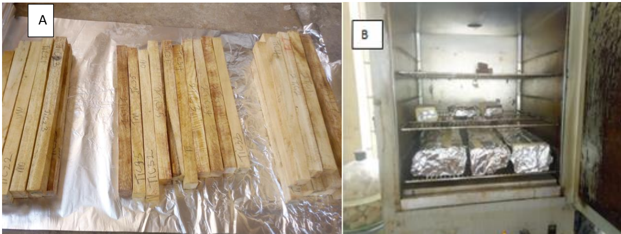
Plate 2: A: Withdrawn Wood samples placed on aluminium foil; B: Curing Processing in Oven.
