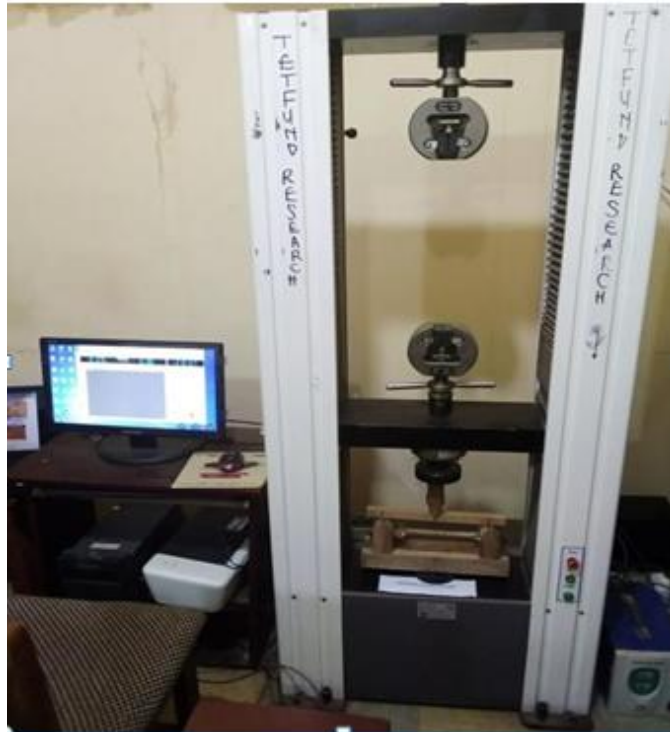
Plate 4: Universal Testing Machine.
