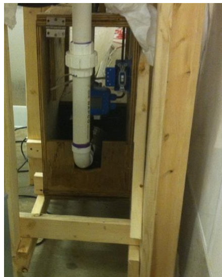
Figure 15: Supercharging pump inlet plenum inside the reservoir elevation frame in the second and final configuration of the coolant recirculation system for the USDA-ARS Farm Animal Behavior and Well-Being Laboratory (FABL) swine calorimetry experiments.
