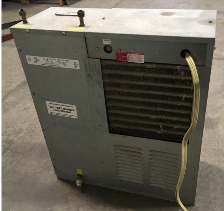
Figure 16: Zurn Elkay ER10 1E (Milwaukee, Wisconsin) water chiller used to thermally recondition the system's coolant and reject the sows' heat to the environment during the swine calorimetry experiment.
