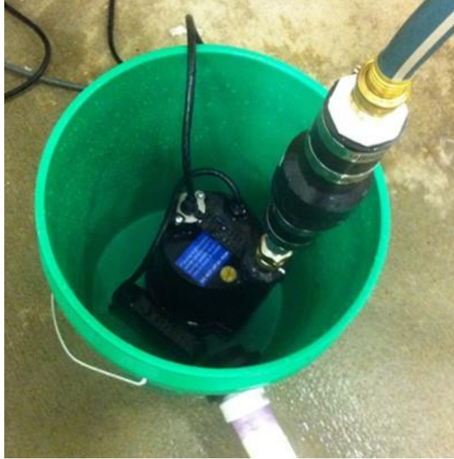
Figure 12: Sump, scavenge pump, and check valve used to return spent coolant to the reservoir during the swine calorimetry experiment at the USDA-ARS Farm Animal Behavior and Well-Being Laboratory (FABL) animal holding room.
