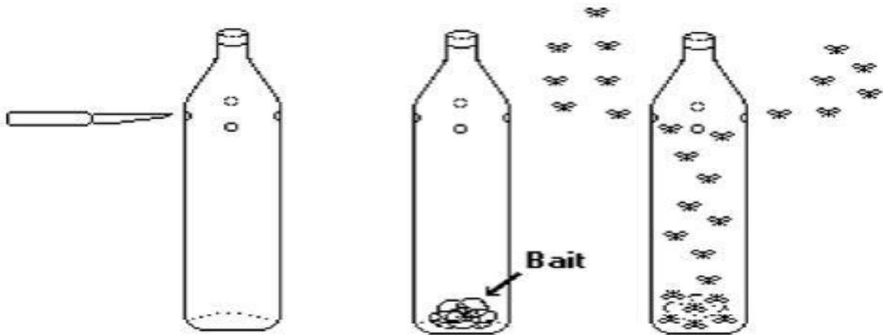
**Figure 2.** Plastic water bottle fly trap (multi-hole model).
