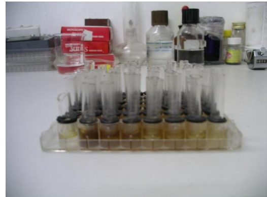
Photo 3. Eight mm glass tubes were kept stand on 48 well-plates by the rubber circles.
