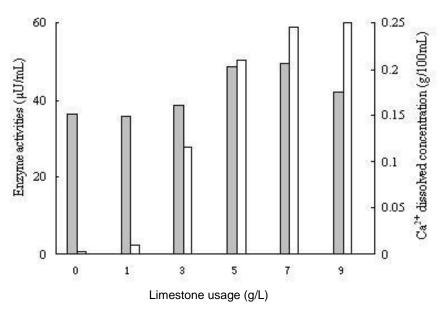
**Figure 1.** Supplied limestone was beneficial for *B. mucilaginous* K02 to synthesize CA. Enzyme activity ( $\blacksquare$ ); Ca<sup>2+</sup> ion dissolved concentration ( $\square$ ). *B. mucilaginous* KO<sub>2</sub> was cultured at 32°C for 6 days.
