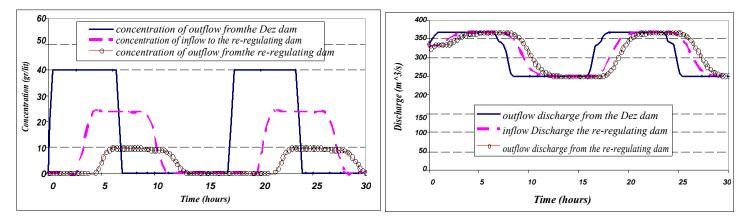
Figure 3. Hydrograph of flow and sediment concentration of the Dez River for the option G2-40 30 based on the model results.
