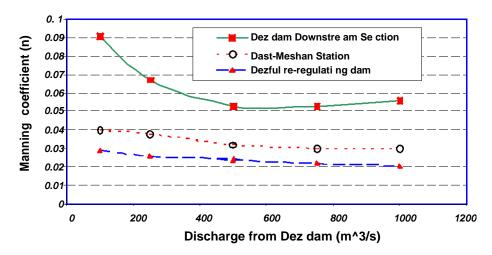
Figure 2. Calibrated Manning coefficient values via discharge in Dez River.
