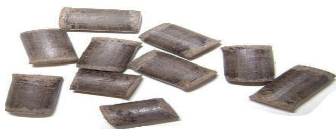
Figure 2. Produced pellets manures from single pelleter setup.
