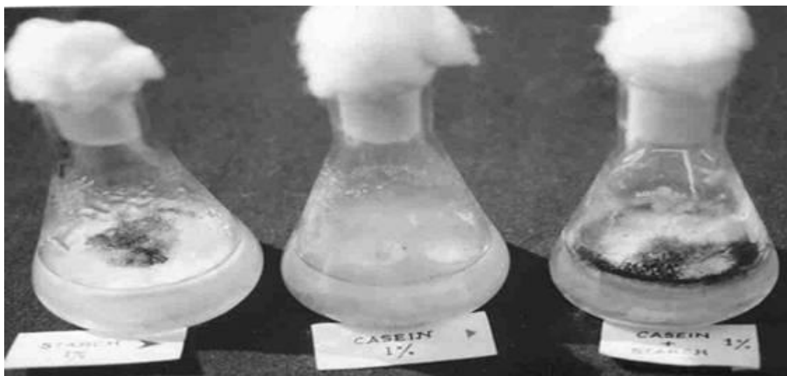
Figure 11. Effect of media engineering on the production of amylase and protease. (1% starch) (1% casein) (1% starch + 1% casein).
