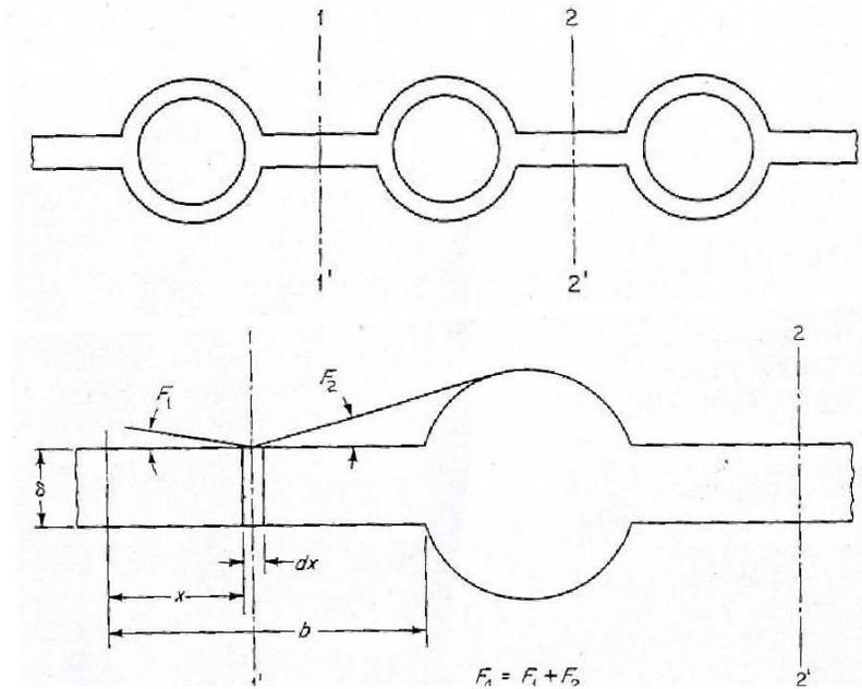
Figure 1. Longitudinal fin-radiator configuration.
