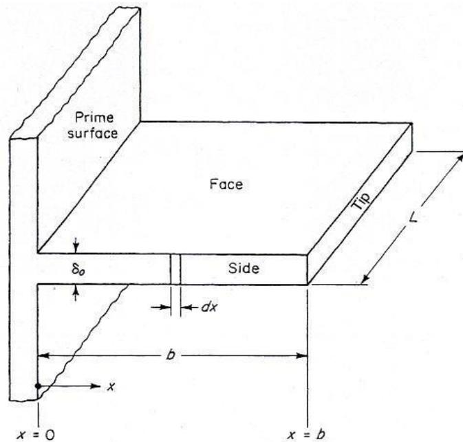
Figure 2. Terminology and coordinate system for a radiating longitudinal fin of rectangular profile.
