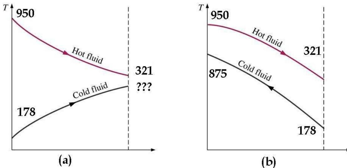
Figure 6. Temperature profile for (a) Parallel flow (b) Counter flow.
