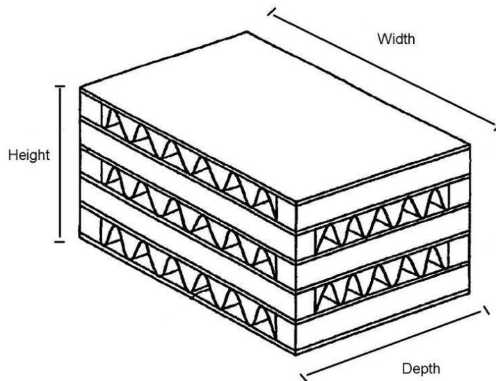
Figure 4. Plate-fin heat exchanger.
