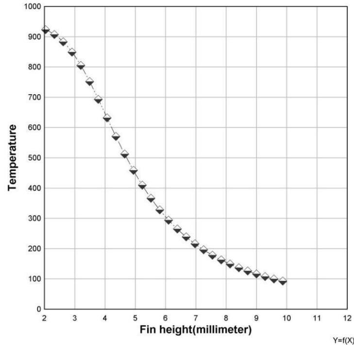
Figure 5. Temperature profile of strip fins for cold stream.
