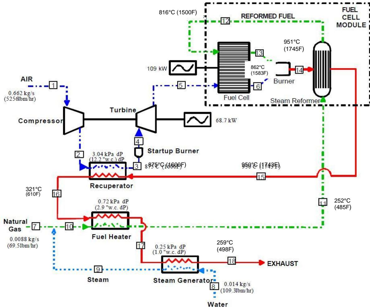
Figure 3. Microturbine cycle (180 kw) (Larry et al., 1990)
