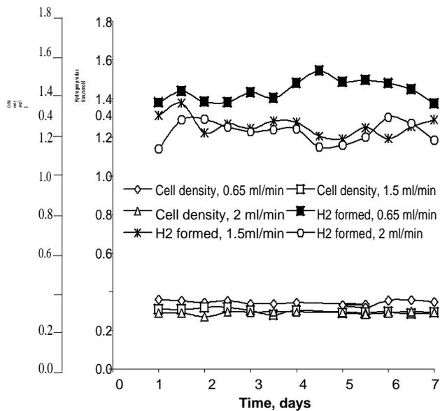
**Figure 4.** Effect of fresh media flow rate on hydrogen production and cell density in continuous fermentation.
