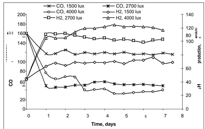
**Figure 6.** Effect of light intensity on H<sub>2</sub> production and CO reduction with continuous culture.
