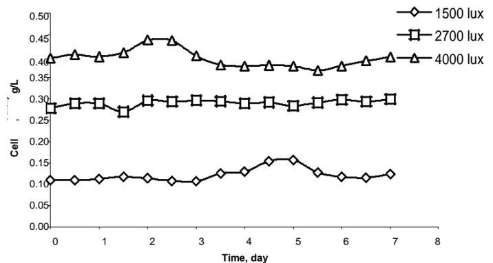
**Figure 5.** Effect of light intensity on cell density in continuous fermentation
