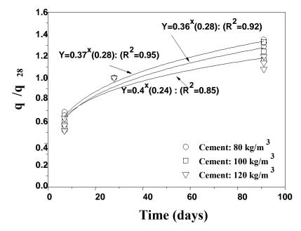
Figure 6. Strength ratio of the CSG material.
