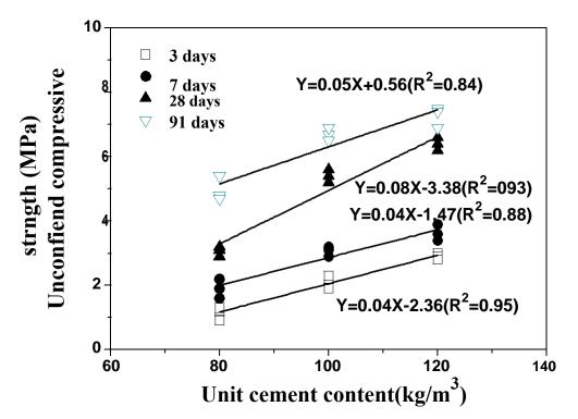
Figure 5. Compressive strength of the compacted CSG material.
