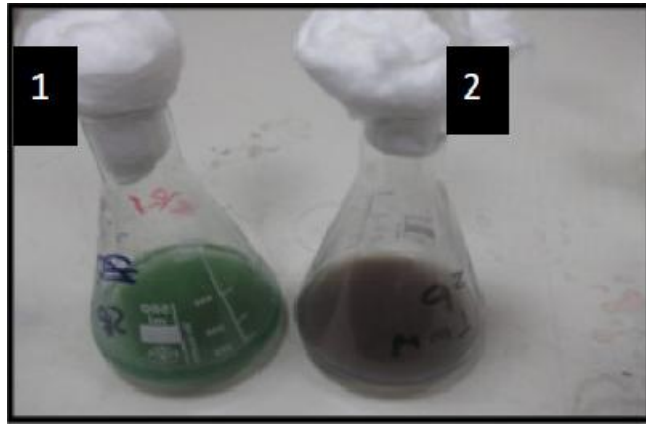
Figure (1): a) the conversion of silver nitrate to nano silver by Spirulina platensis biomass. The picture shows the growth of Spirulina platensis in Zarouk's medium (1) and the color changes (2).
