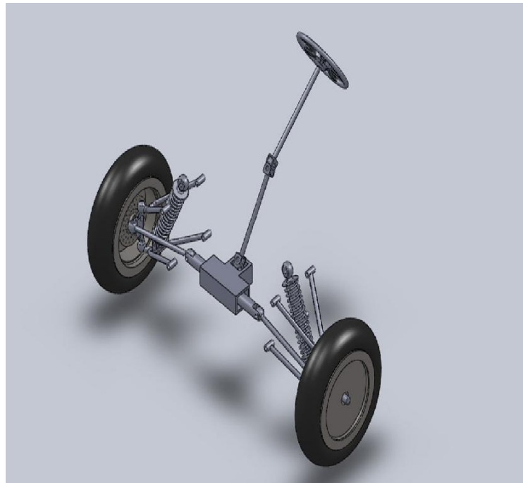
Figure 5. Rack and Pinion aided Ackermann steering system.
