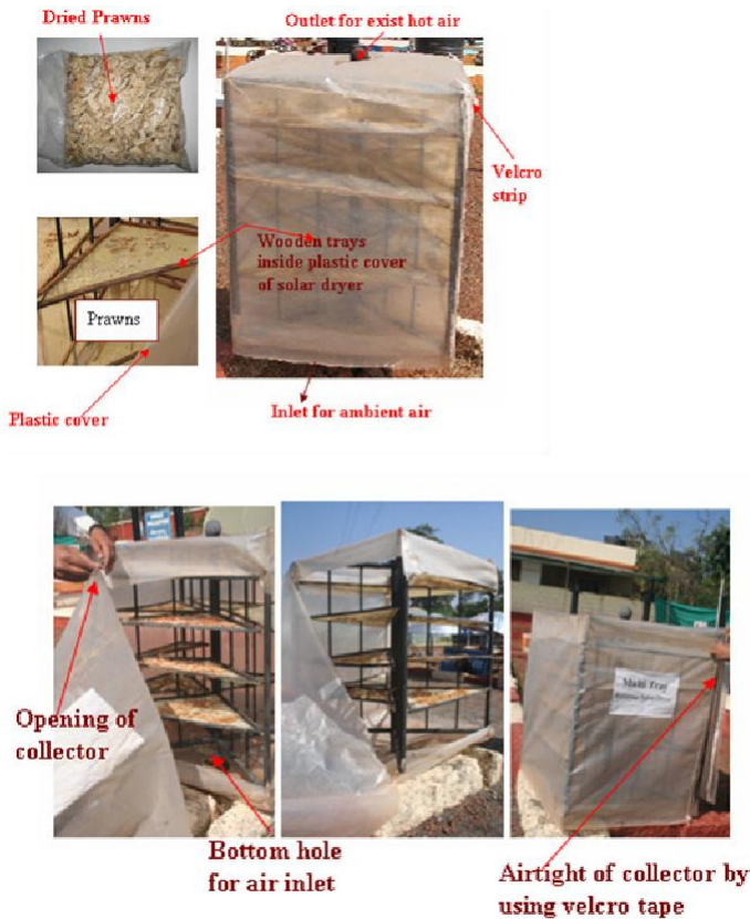
Figure 2. Vertical rotary low cost solar dryer.
