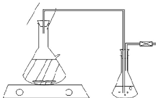
**Figure 1.** Anaerobic fermentation system for ethanol production.
