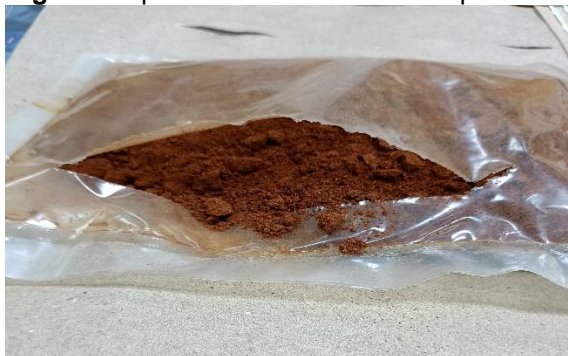
Best results were observed in Paper woven Bag with Liner IV (PA/EVOH/PE – 9 Ply; 70- 80 \mu )
