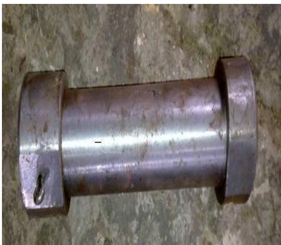
Figure 4. Longitudinal crack in cage pin with nut.
