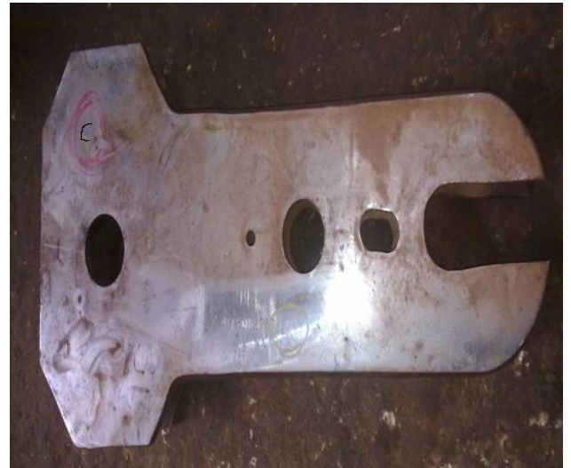
Figure 5. Complex type crack in rivet of outer plate of safety hook
