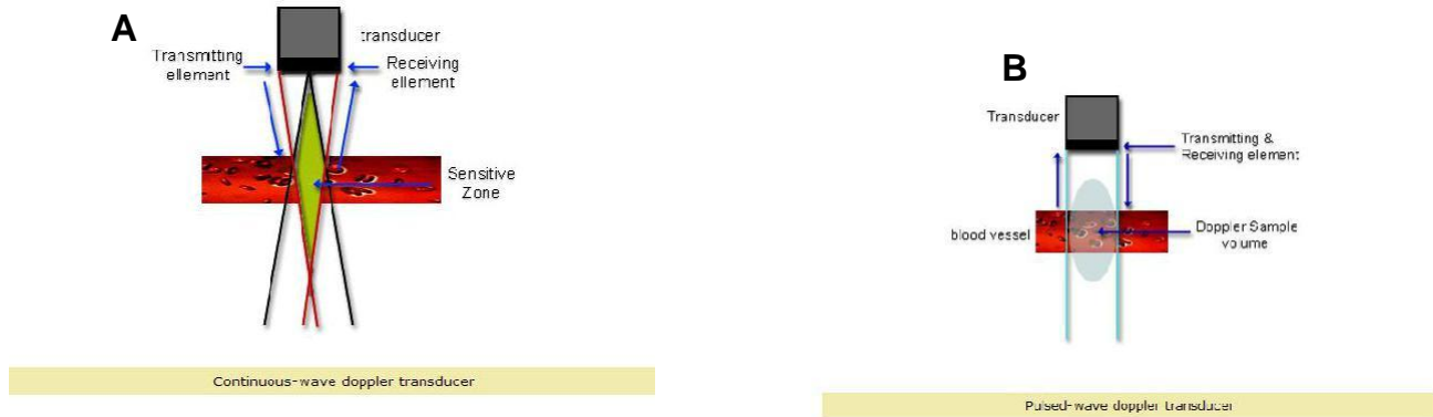
Figure 1. Comparisons of two types of Doppler systems, a and b.
