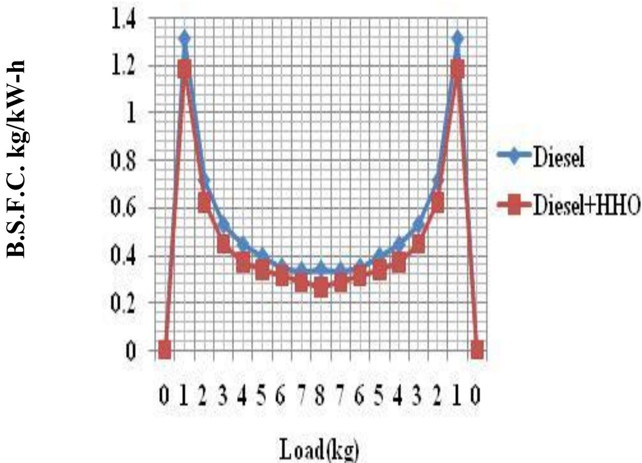
Figure 6. Graph of brake specific fuel consumption in kg/kW-h v/s load in kg.
