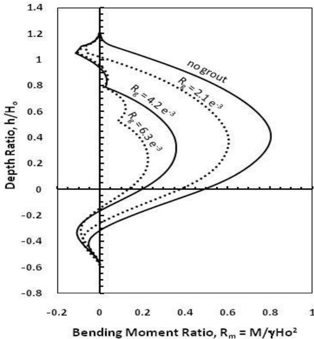
**Figure 3.** Bending moment ratios,  $R_m$  along sheet-piling quay wall due to various values of grouting area ratio,  $R_g$ .
