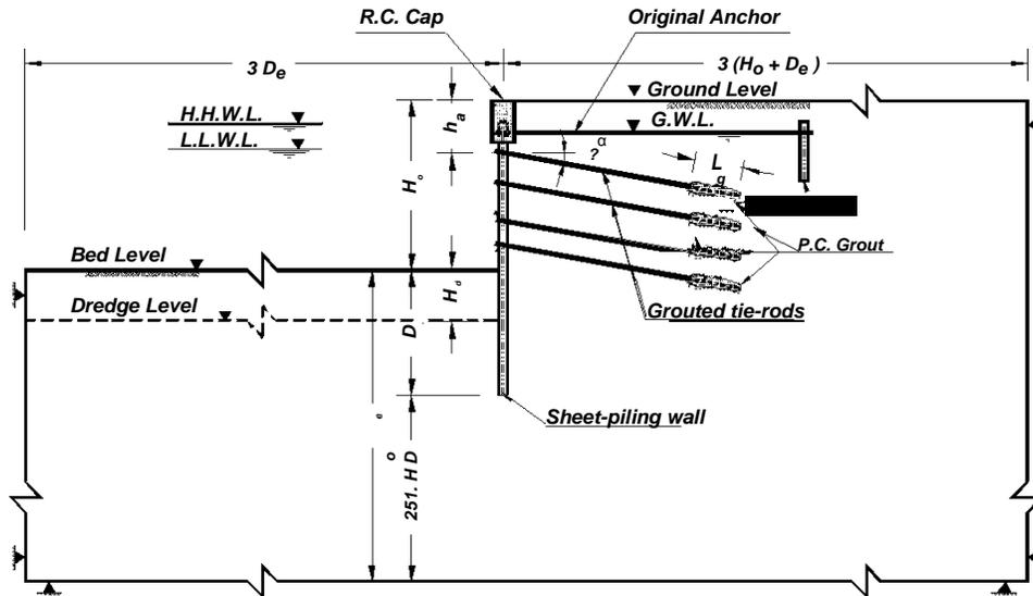
Figure 1. Geometry of Multi-Anchored-Sheet Pile System.
