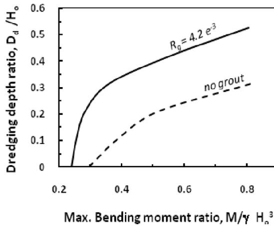
**Figure 11.** Maximum bending moment ratio,  $R_m$  versus dredging depth ratio,  $R_d$ .
