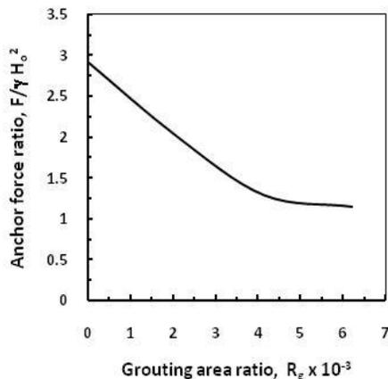
**Figure 6.** Anchor force ratio,  $R_F$  due to various values of grouting area ratio,  $R_g$ .
