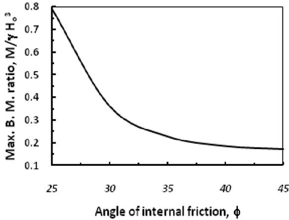
**Figure 7.** Maximum bending moment ratio,  $R_m$  versus backfill soil angle of internal friction,  $\phi$ .
