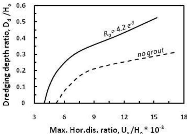
**Figure 13.** Maximum horizontal displacement ratio,  $R_{ux}$  versus dredging depth ratio,  $R_d$ .
