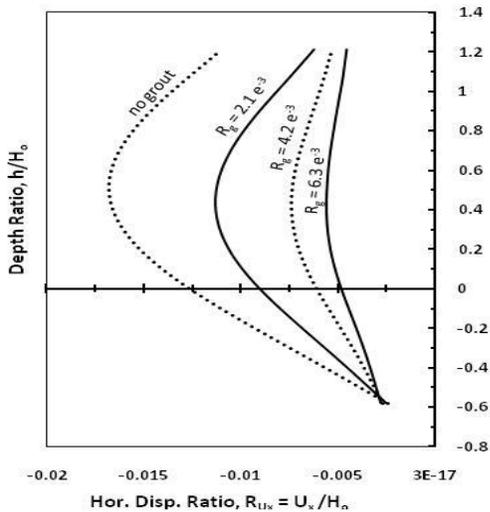
**Figure 4.** Horizontal displacement ratios,  $R_{Ux}$  along sheet-piling quay wall due to various values of grouting area ratio,  $R_g$ .
