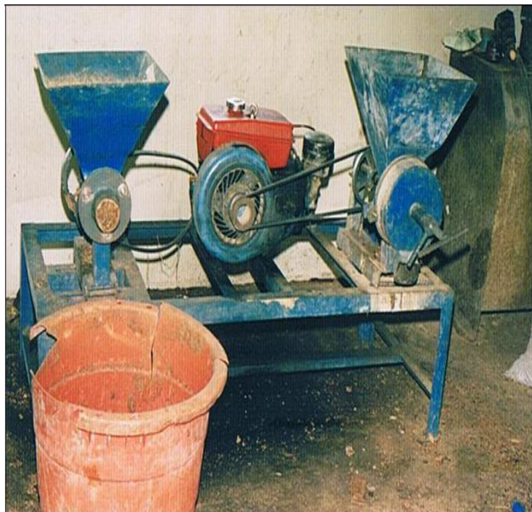
Figure 1a. Locally Fabricated diesel pelleting machine.
