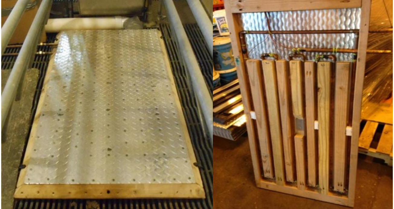
Fig.3. Exterior of the second prototype (eight-pipe) Purdue hog cooling pad installed in a farrowing crate at the Purdue Animal Sciences Research and Education Center (left), and the operational interior of the same unit showing cooling coil layout (right).
