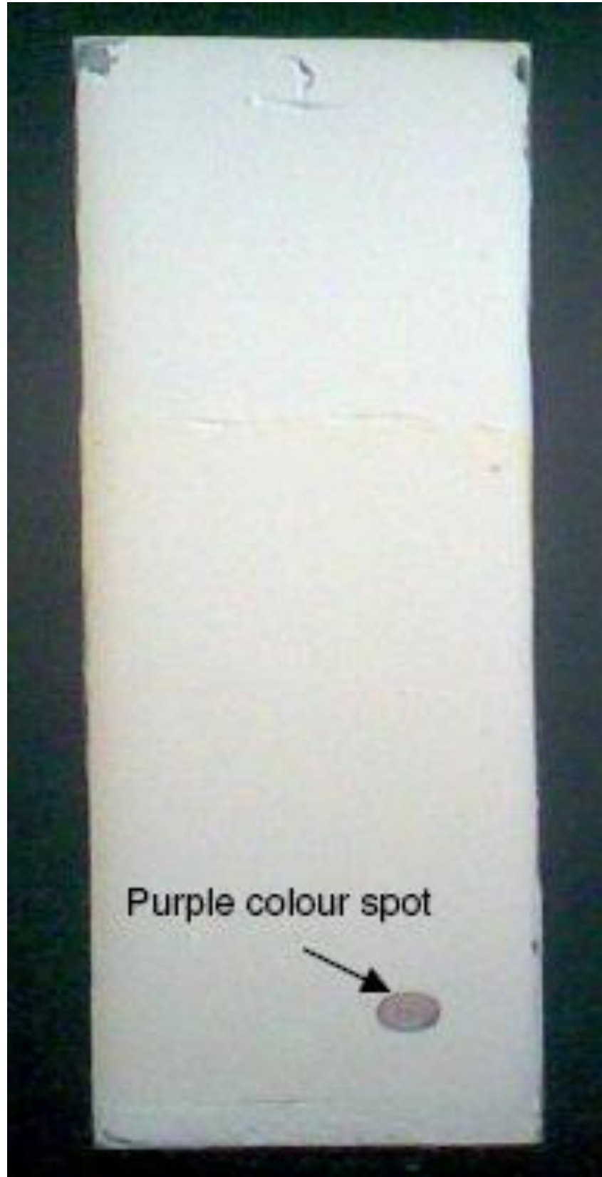
Figure 2. Thin layer chromatogram in Merck silica gel 60 F 254 showing a characteristic purple blue spot in the area of spotting the crude endophytic fungal metabolic extracts (RS07PF) upon exposing the TLC plate to iodine vapours.
