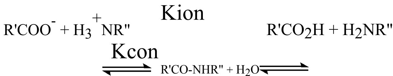
Figure 3. K_{ion} is the equilibrium constant of ionization and K_{con} is the equilibrium constant of conversion.
