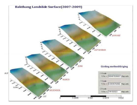
Figure 6. Surface formed by GPS periodic data of the landslide.
