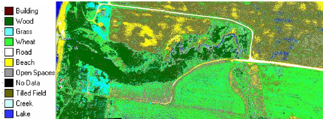
Figure 3. Pixel-based classification results of airborne Infrared image based on Maximum likelihood classifier, Eastern shore of Lake Huron, Ontario, Canada.
