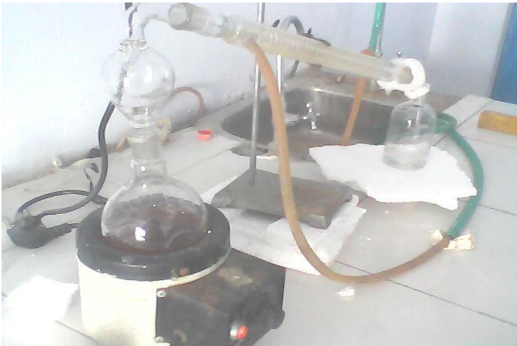
Figure 2. Production of bioethanol in a condenser apparatus.
