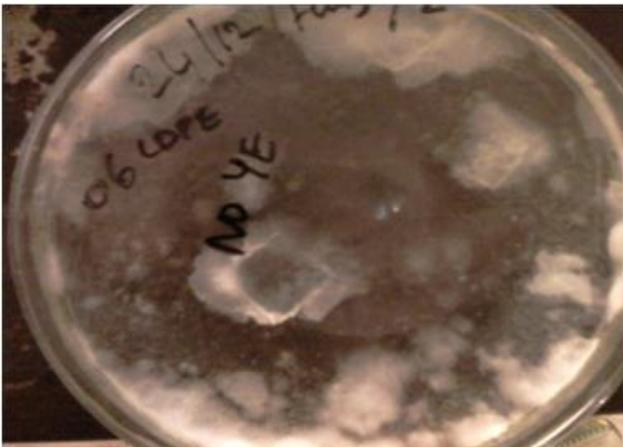
**Figure 2.** LDPE film showing colonization of hyphae.
