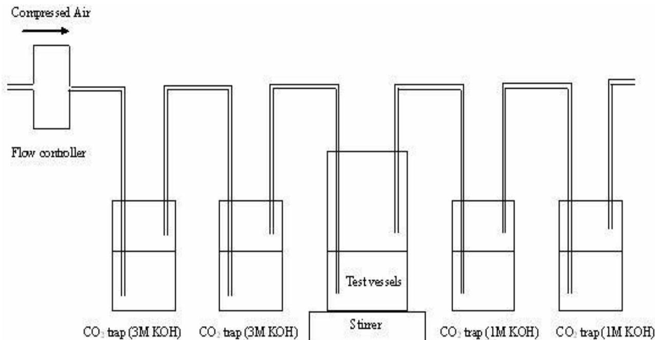
Figure 1. Sturm test.
