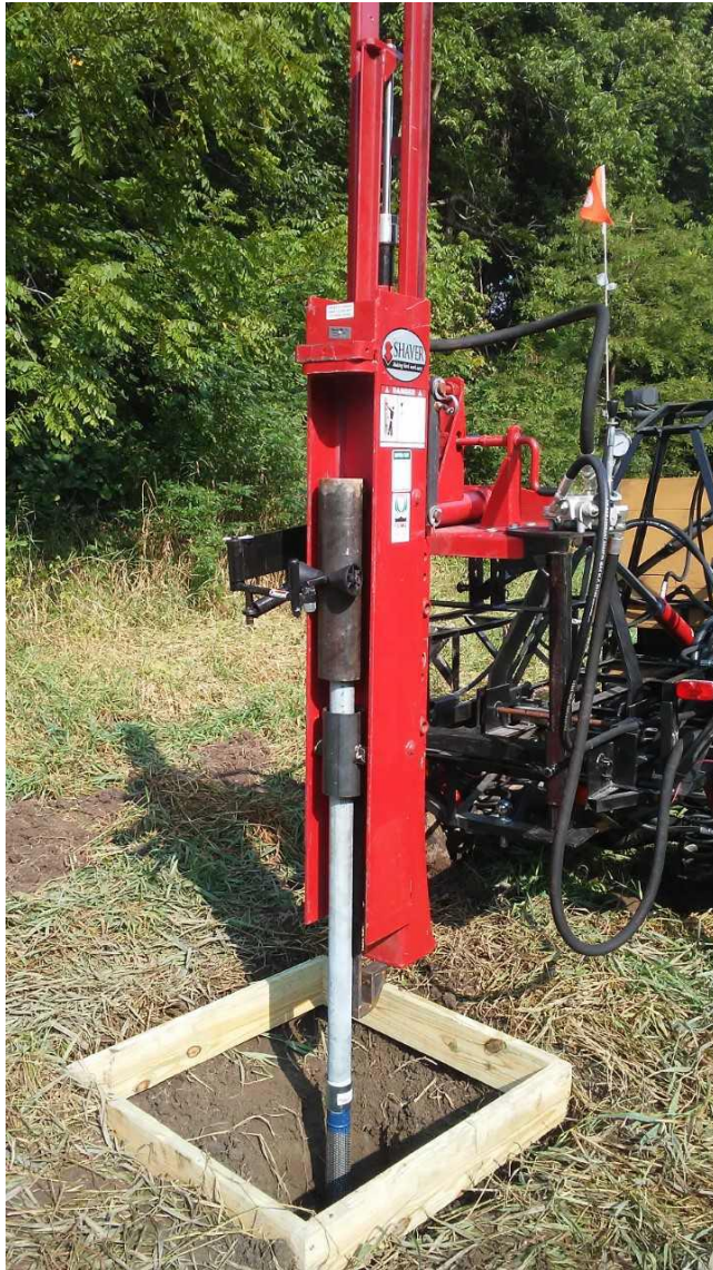
Figure 2. Well Driver PUP in position over a test well in west-central Indiana during proof-of-concept tube well mechanization experimentation on the left and cross-section of driven well showing well point and drive joints couplings on the right.
