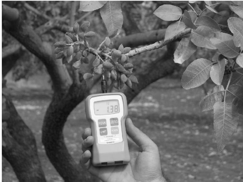
**Figure 2.** Measurement of fruit detachment force.
