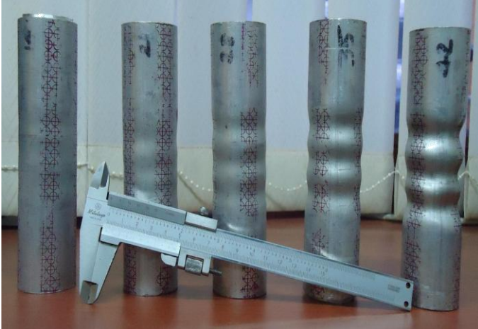
Figure 3. Roll forming compression test at different levels of pressure.
