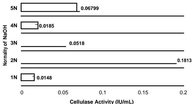
**Figure 1.** Effect of NaOH pretreatment on *Aspergillus niger* cellulase activity using saw dust as substrate.
