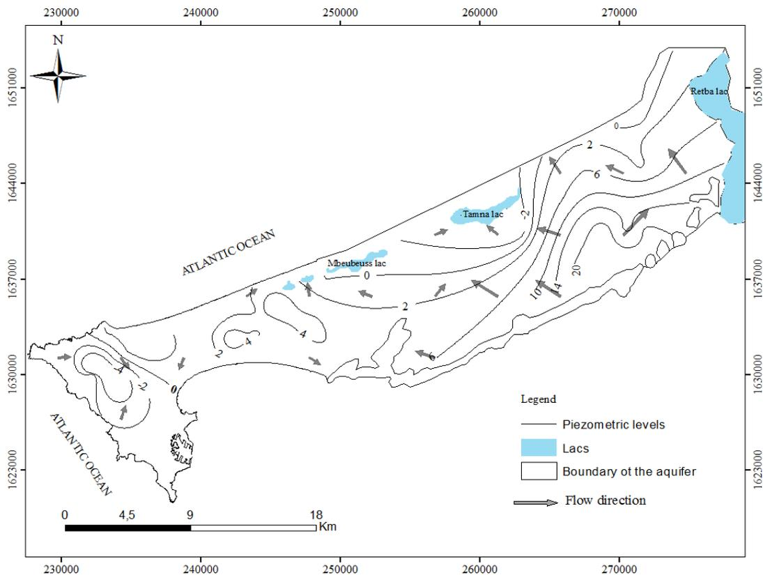
**Figure 3.** Piezometric map (mars 2008).
