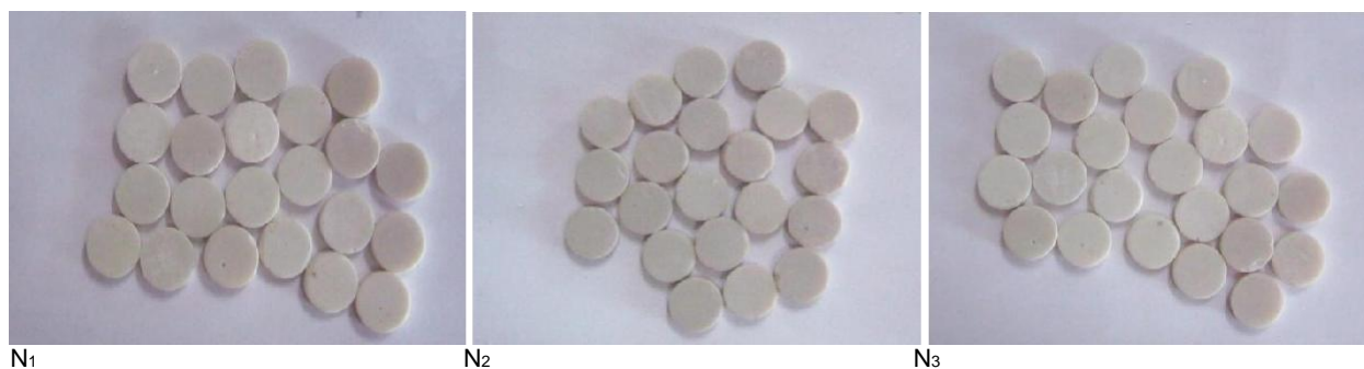
Figure 2. Indomethacin tablets formulated with lipid matrix ratio (SRMS) 1:1, 2:1 and 1:2 (N 1 , N 2 , and N 3 ), respectively.
