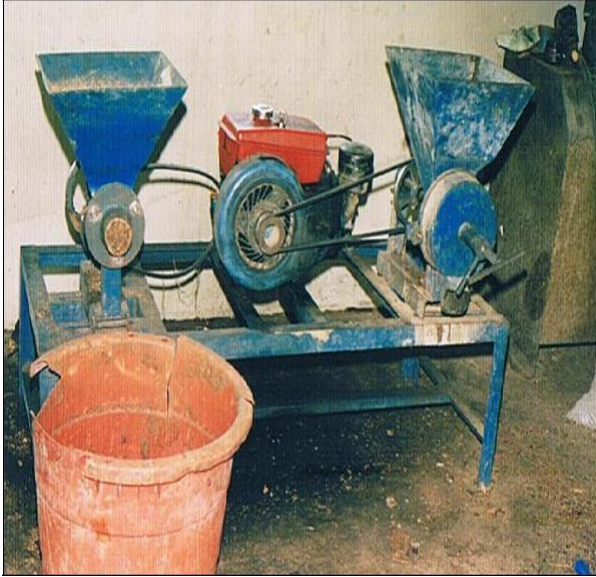
Figure 1a. Locally Fabricated diesel pelleting machine.
