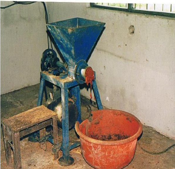
Figure 1b. Locally Fabricated electric pelleting machine
