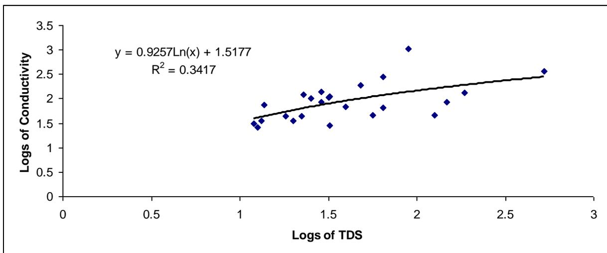
Fig 4. Regression between Logs transformed Conductivity and TDS at Site III in River Benue at Makurdi.
