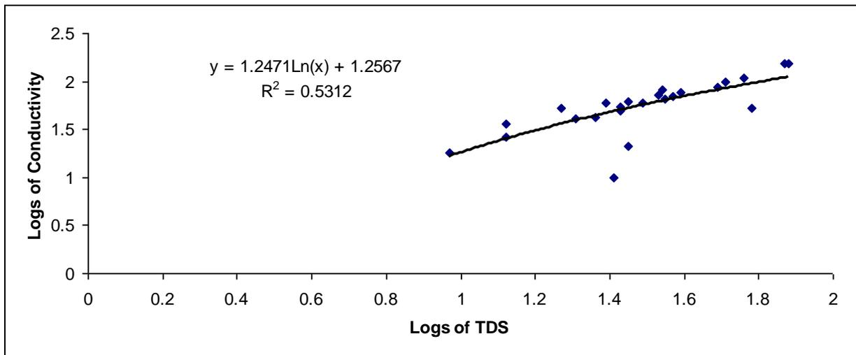
Fig 2. Regression between Logs transformed Conductivity and TDS at Site I in River Benue at Makurdi.
