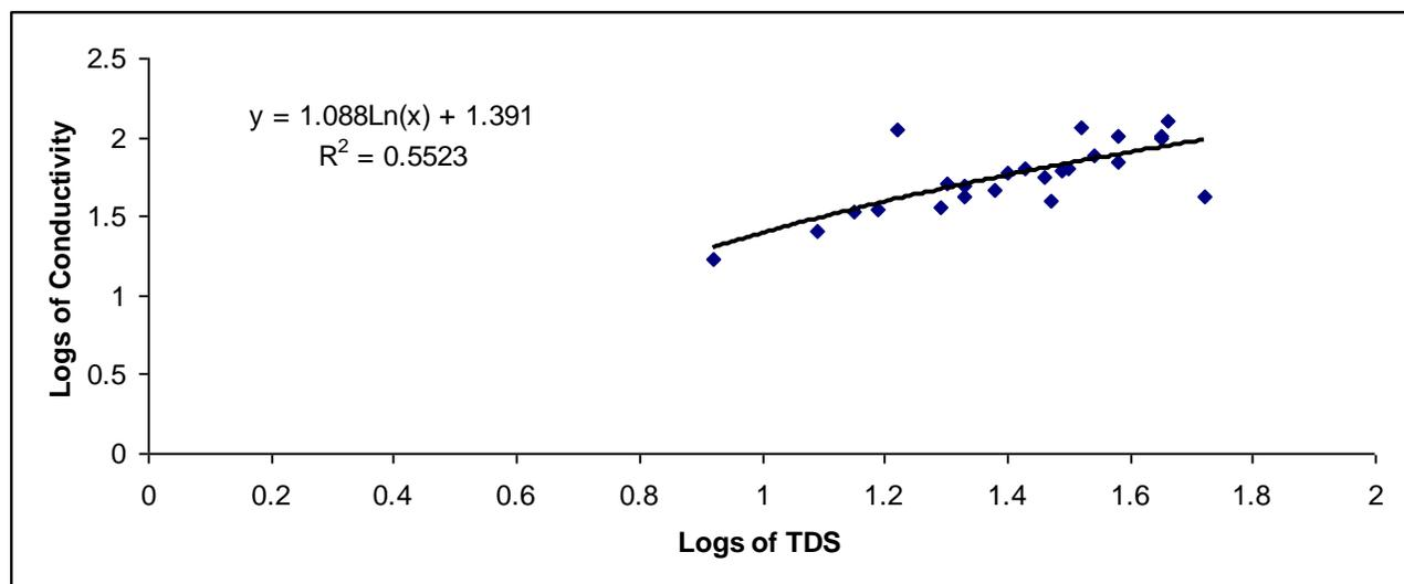
Fig5. Regression between Logs transformed Conductivity and TDS at Site IV in River Benue at Makurdi.
