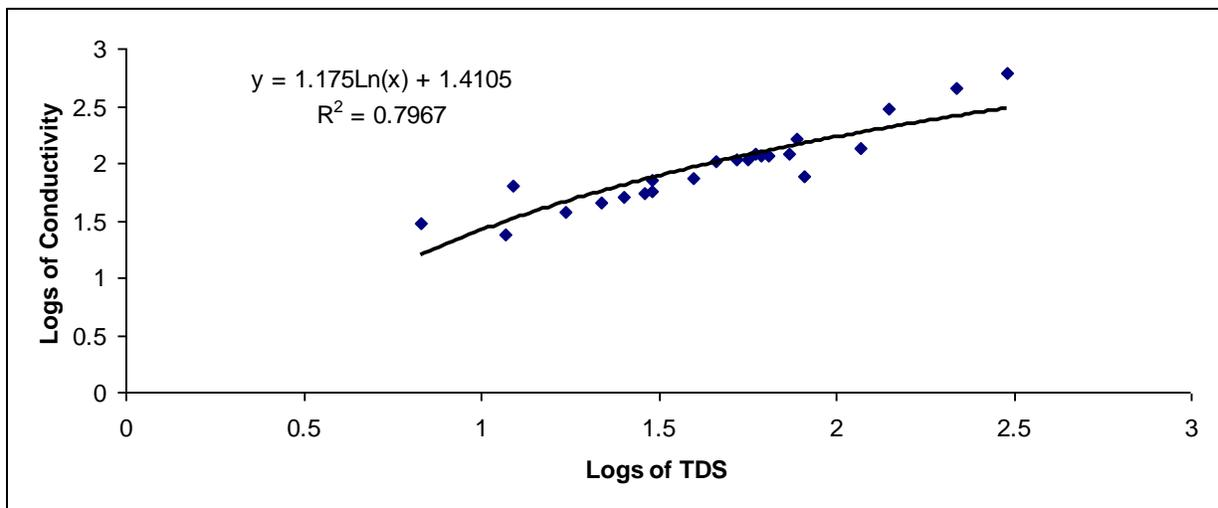
Fig 3. Regression between Logs transformed Conductivity and TDS at Site II in River Benue at Makurdi.
