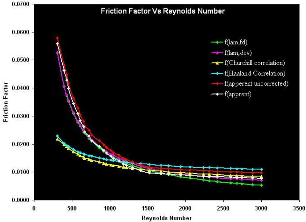
Figure 3. Comparative plots of friction factor with the experimental results.
