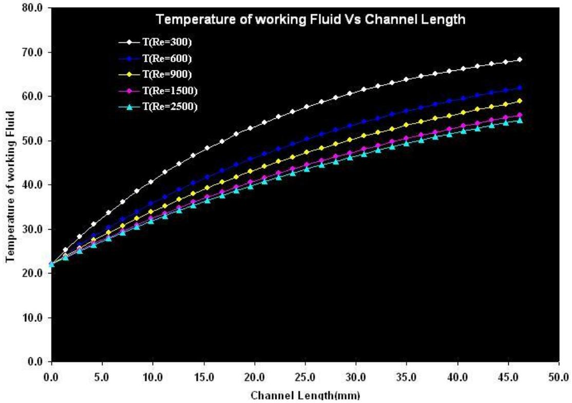
Figure 7. Temperature profile of working fluid along the channel length for different Reynolds number.
