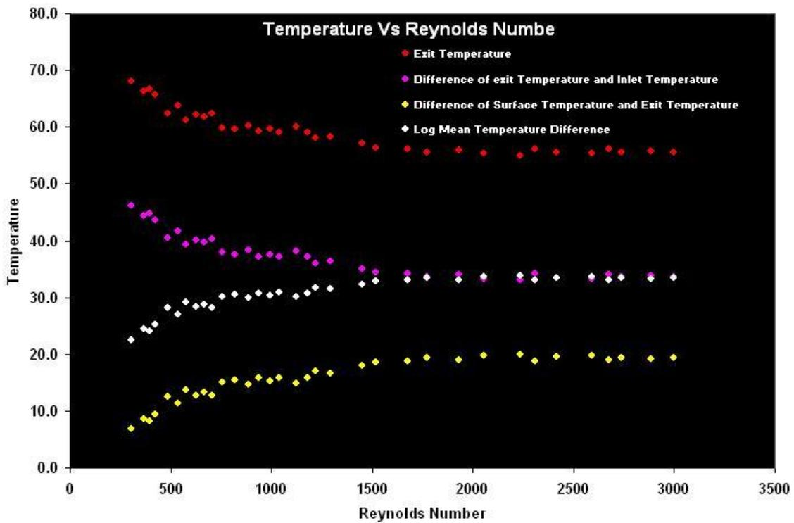
Figure 5. Temperature profiles of w.r.t. Reynolds number.
