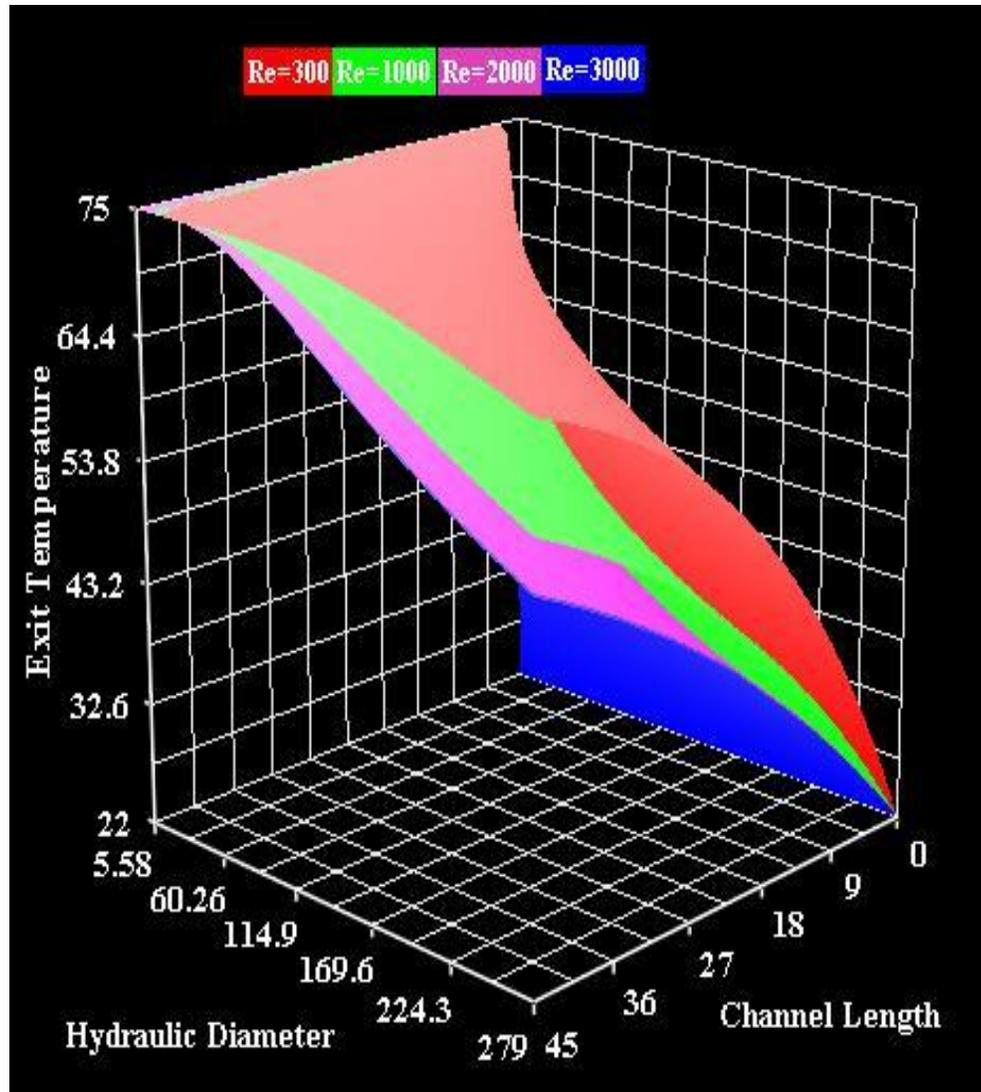
**Figure 9.** Surface plots of temperature profile of working fluid along as well as across the channel for different Reynolds number.
