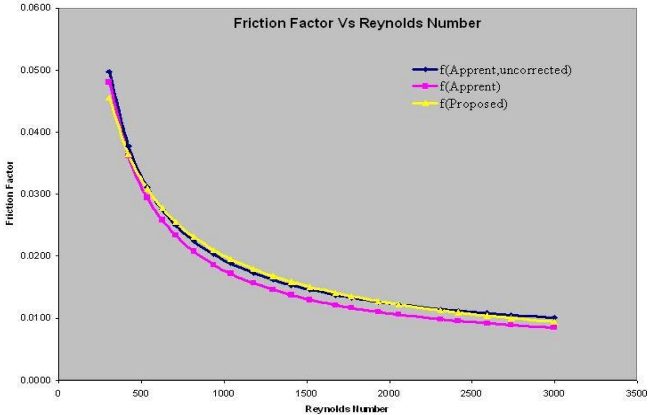
Figure 4. Comparative plots of experimental friction factor with proposed equation.
