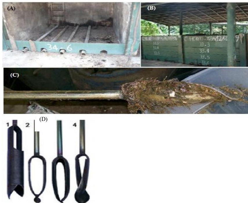
Figure 2. Large-scale cell composting at UPCO. (A) empty composting cell; (B) front view of two composting cells; (C) auger containing compact compost; (D) manual kit of Eldeman's auger (Eijkelpark Agrisearch Equipment, Giesbeek, Netherlands): Type 1, riverside auger - for the coarse sandy soils and little mixed cohesive (between 35 to 40 cm in length); Type 2, Edelman auger for clay and cohesive soils (between 25 to 30 cm in length); Type 3, Edelman auger for sandy soils and non-cohesive (25 to 30 cm in length) and Type 4, Edelman auger for very dry sandy soils with little or no cohesion (between 25 to 30 cm in length).
