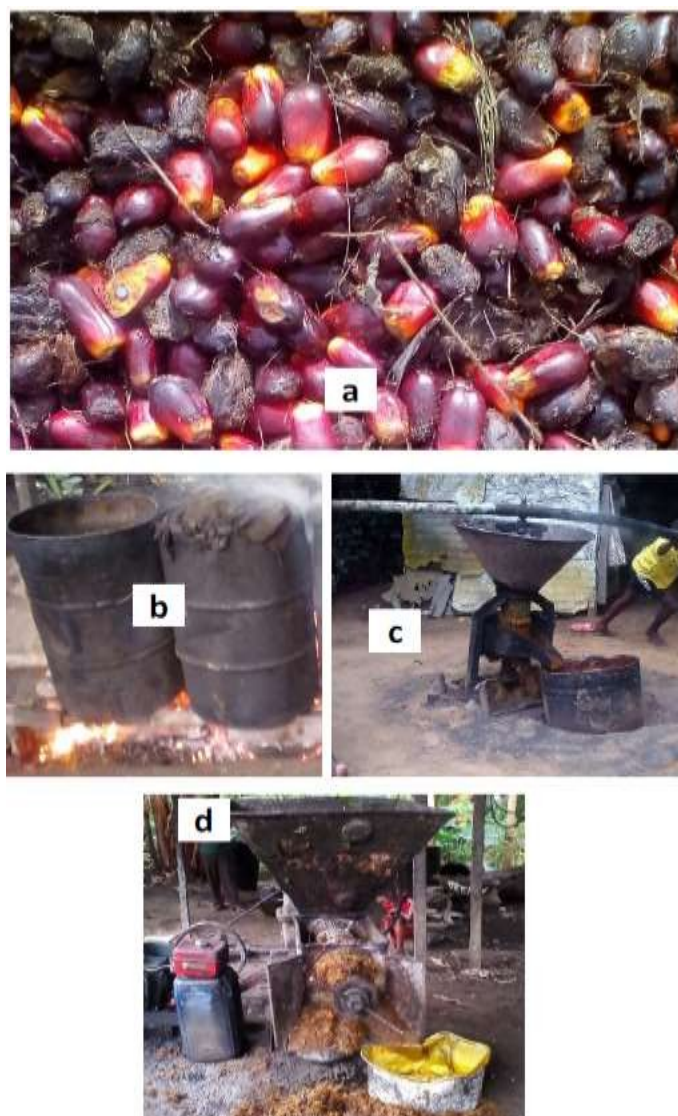
Figure 2. Some materials used by smallholders for artisanal palm oil production in Cameroon; a: fruits stored for several days; b: boiling of fruits with inappropriate apparatus; c: 'round the world' press and d: motorized press.
