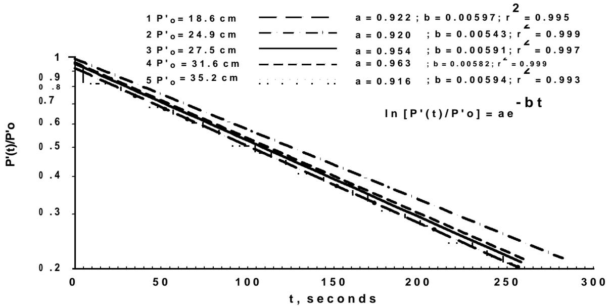
**Figure 3.** Semi-logarithmic plots for fitting the two-parameter equation  $P(t)/P_o = ae^{-bt}$  to a truncated set of data points for  $P'(t)/P'o$  versus time (t) measured for the 5 values of  $P'o$ .
