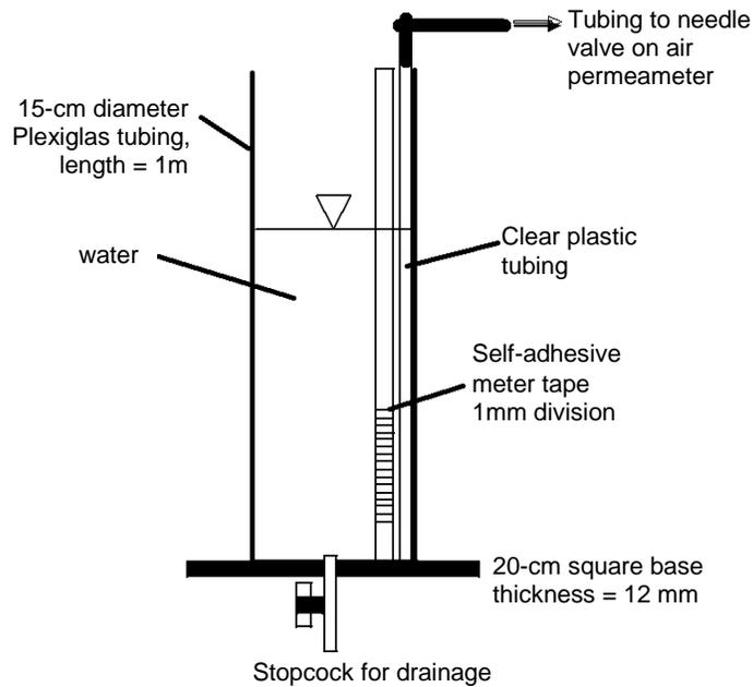
**Figure 2b.** Pressure regulator and manometer assembly.
