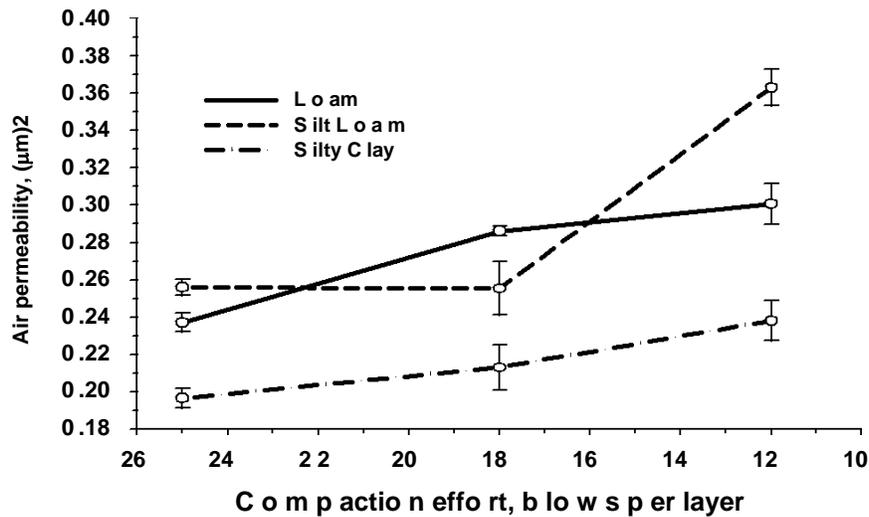
**Figure 4.** Air permeability (estimated using the two-parameter fitting equation  $P(t)/P'o = ae^{-bt}$ ) with decreasing compaction effort. Error bars represent the standard error of the mean of 5 repetitions on a given test specimen.
