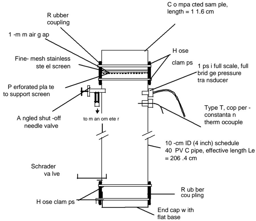
**Figure 2a.** Air permeameter chamber assembly.
