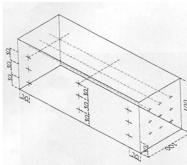
**Figure 1.** Measuring points of inner compost temperature
