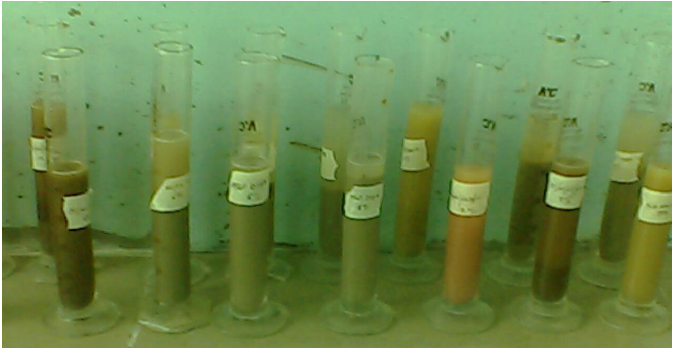
Figure 5. Free swell volume determination.
