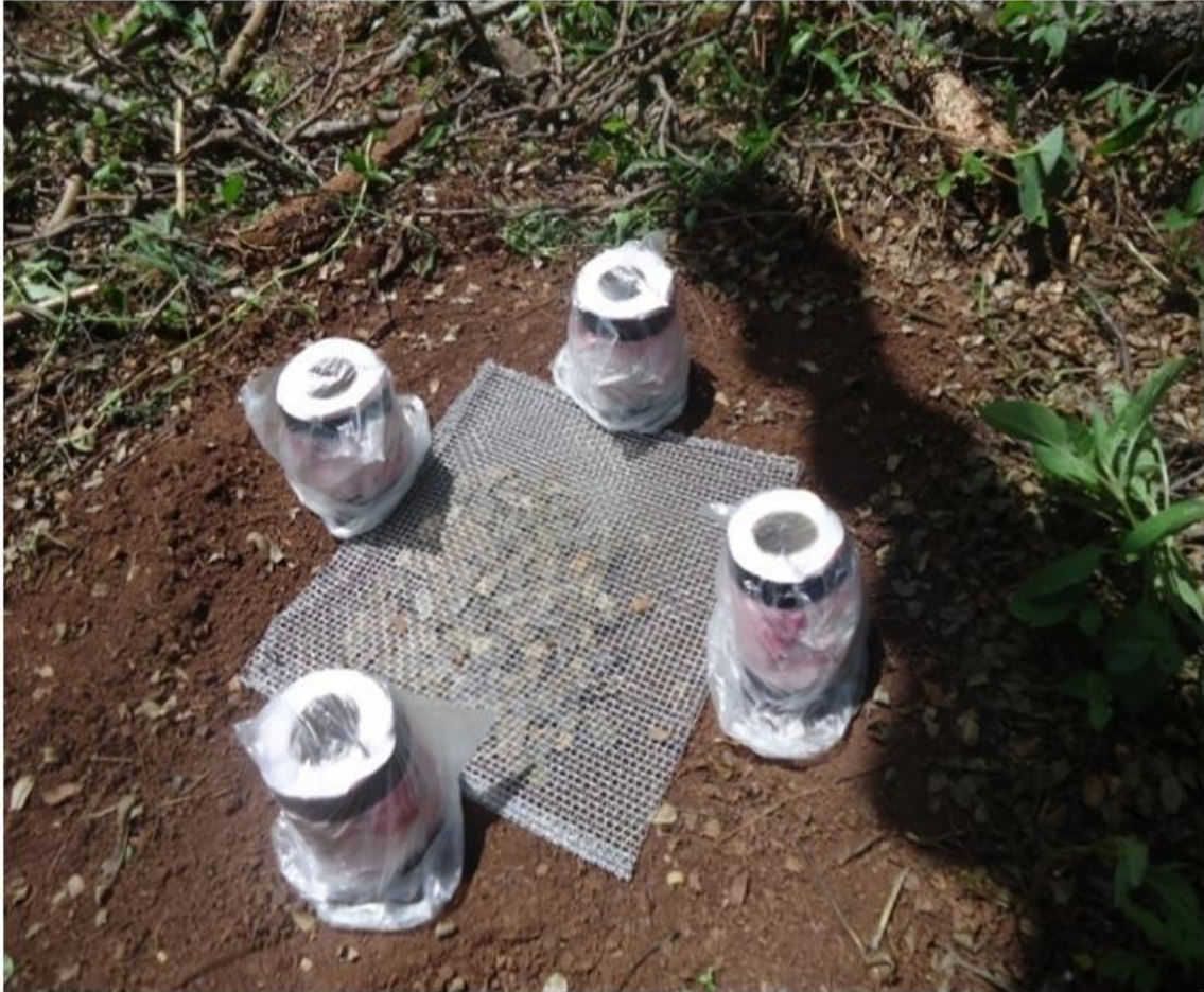
Figure 1: Tissue paper roll baits for sampling termites placed around a litterbag
